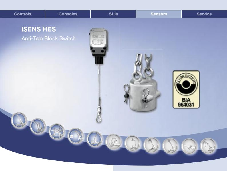
iSENS HES is a positive opening limit switch for safe upwards movement of the hook. The anti-two block switch is used on winches, cranes and lifting equipment. The housing is made of a corrosion-proof, light metal alloy, the surface of which is further treated and coated and as such it is resistant to the damaging affects of the atmosphere.
